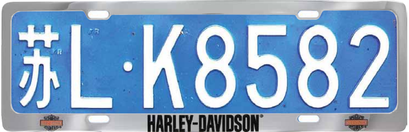
License plate frame dimensions: 447mm x 147mm (HDLF16-CN seen above). China license plate dimensions: 444.5mm x 146.6mm
