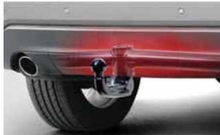
Swan-neck trailer hitch ball attached under typical European vehicle.
